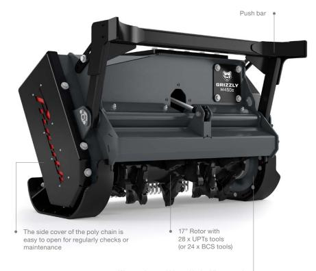
Wear resistant skids and bolted liners made from Hardox to protect the housing
